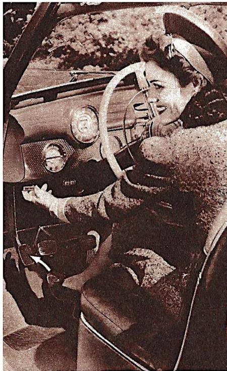
"Step-On" emergency brake, by Buick, operates by foot and has dash release to eliminate "fumbling."
