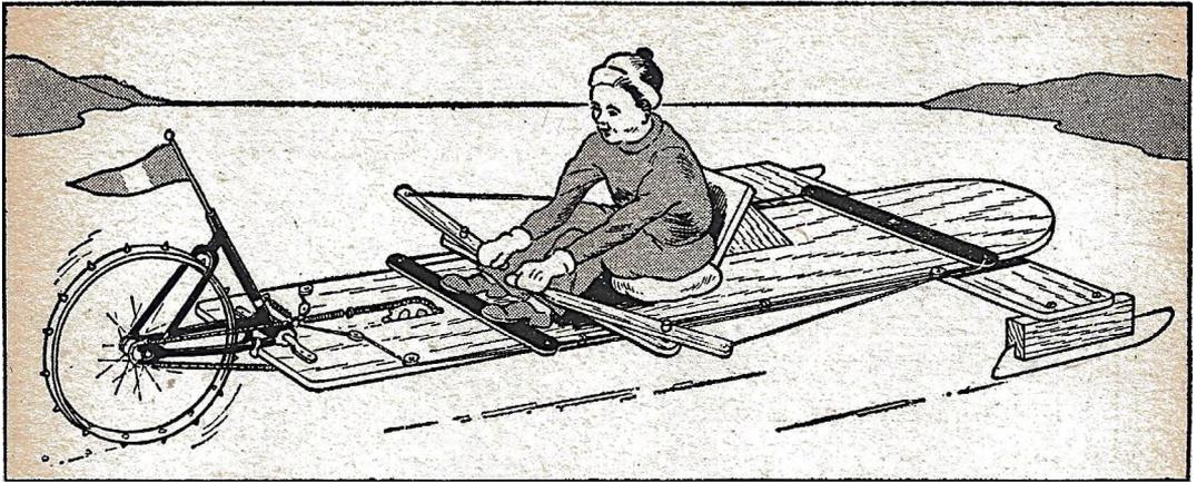
**T**HE platform consists of a simple plank 9 ft. long, 18" wide and 1" thick. Or you can cleat two narrower boards together underneath, making due allowance for fittings, etc. Round off one end for the bow but leave the stern square.
